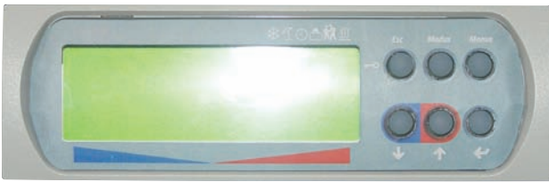
Fig. 3.2: Heat pump controller (HPC) with integrated display
